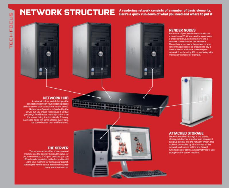
connect your computer to an Ethernet network. Many newer machines will support the fastest 1000BaseT Gigabit standard, which is capable of transferring a 500MB image in less than half a second. That might sound fast, but when you consider that you need to send images back and forth between every machine connected to the network, speed isn't a luxury, but a necessity.
