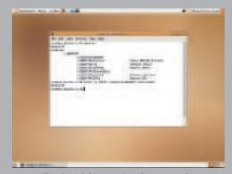
The shared drive needs to be mounted onto your Linux machines so that they can read and write to the same drive. The command for doing this is a little technical, but well documented in Ubuntu. Network storage in Linux appears just like local storage, and will become part of the normal directory tree.
